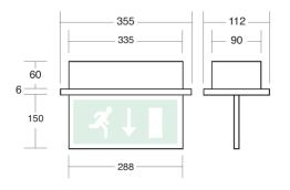
Recessed: the housing has adjustable spring clip arms to simplify installation into different thickness supporting surfaces.
