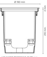
HOLE FOR RECESSING Ø 179 mm
