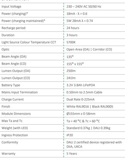
**Note**\* After its initial charge, It will spend 90% of its operational life in standby mode. If DALI is not present the unit will defaults to Self-Test operation.
